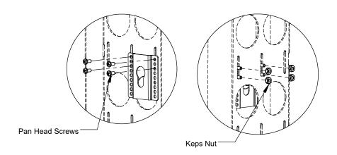
\*NOTE: Correct screw location varies depending on the PDU and the height of the Cable Managment Bar.
