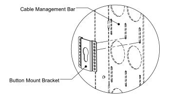
Step 2 Securing the Button Mount Bracket: Install the Pan Head Screws into the appropriate hole location and secure it to the Cable Management Bar with Kep Nuts.
