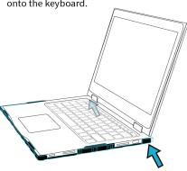
Once successfully installed, open the case by using the center lift tab only!
