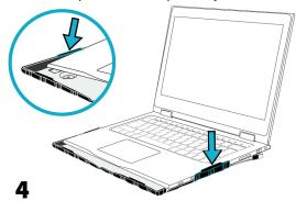
Slide the top case down, to secure the screen behind the side clips, until the device reaches
