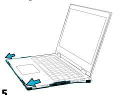
Press the lower side clips over the device, with pressure from both sides, to snap into place securely.
