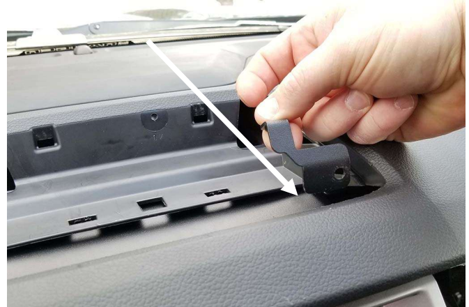
Slide passenger side upper mount bracket ( end with no threaded hole ) down from tray opening and position bracket behind passenger side OEM display mount. Do the same for driver side.
