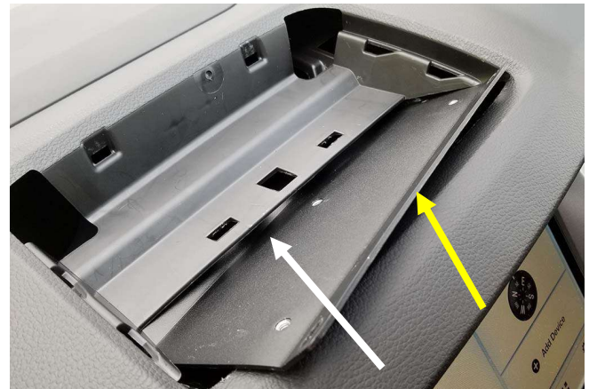
Slide top clamp bracket into the tray opening underneath the plastic cross support.
