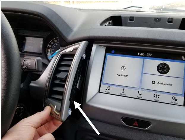
Carefully unsnap and remove driver side vent and trim next to steering column.
