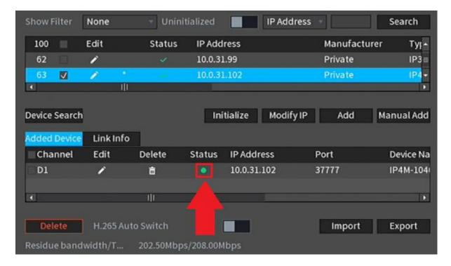
As previously stated, our H.265 compatible products will come **factory defaulted to H.264 compression**, but for increased performance, the camera's settings can be automatically switched to H.265 compression. Switching to H.265 compression reduces bandwidth **without sacrificing frames per second or resolution**. To activate H.265 compression, click on the **H.265 Auto Switch**.
