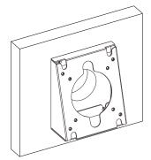
Fix enclosure or screen on the mount using 4pcs M5\*10 screws.
