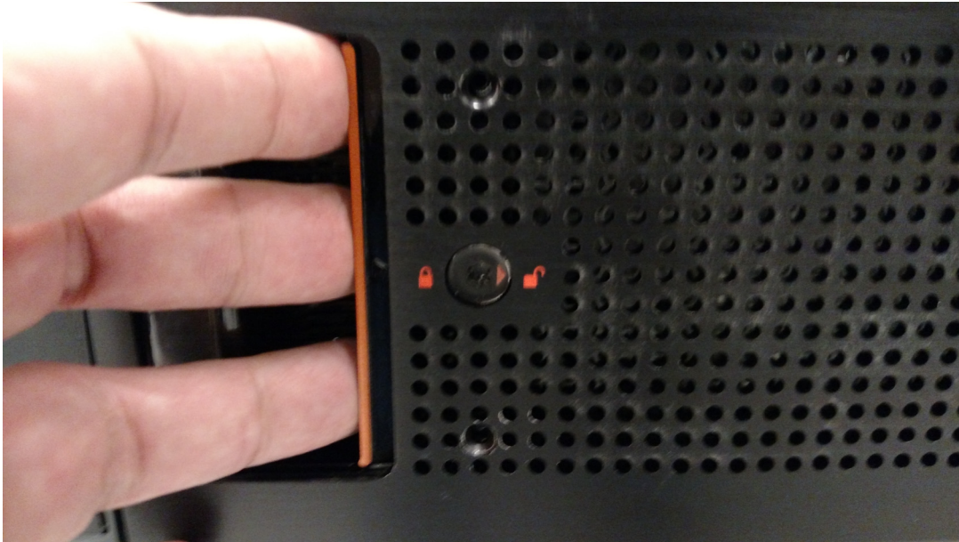
Figure 158 5U84 Chassis Bezel Drawer Latches (2 Each)
