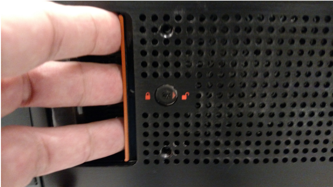
Figure 162 5U84 Chassis Bezel Drawer Latches (2 Each)
