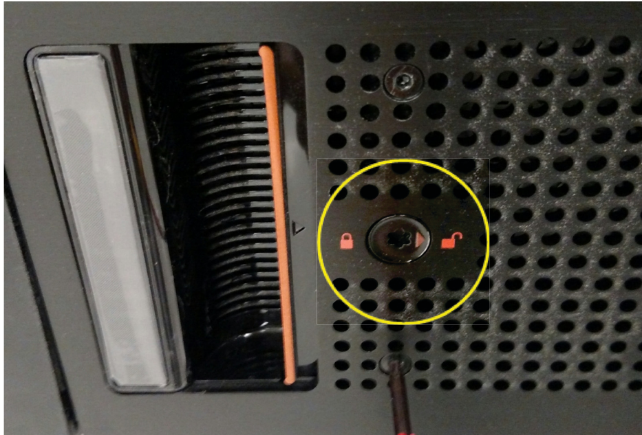
Figure 157 5U84 Chassis Bezel Screws (4 Each)
