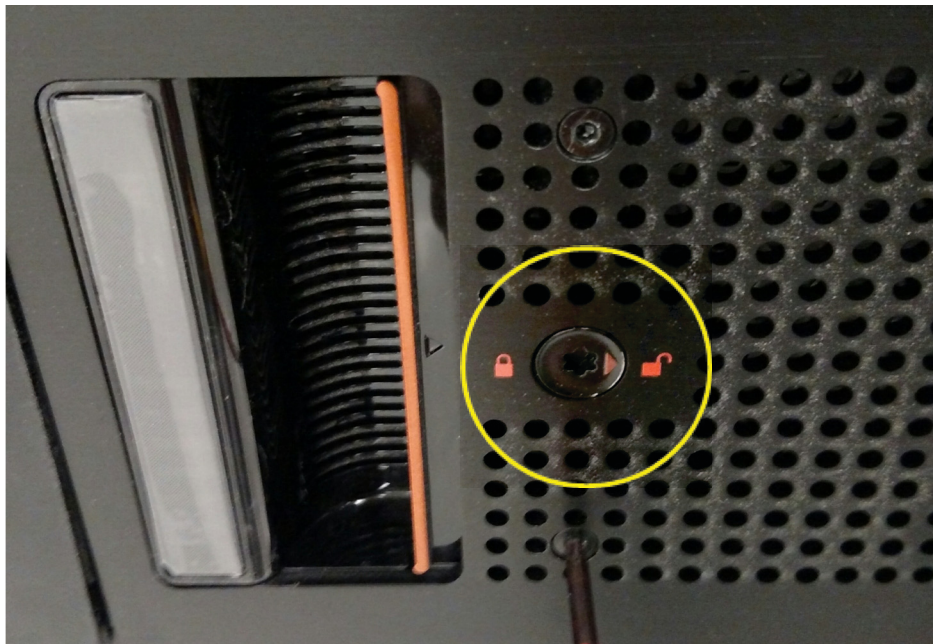
Figure 161 5U84 Drawer Unlock Anti-tamper Locks
