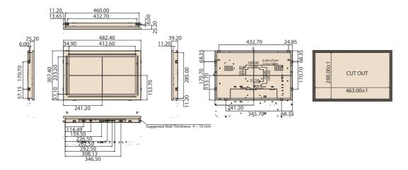
Figure 2.1 IDS-3218WG/IDS-3218WR Dimensions
