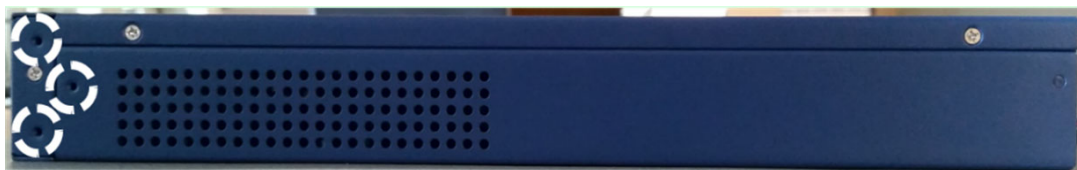
Figure 1.1 Mounting ear thread holes
