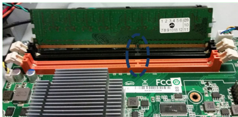
Figure 3.42 DIMM key alignment
