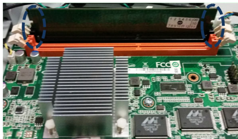
Figure 3.43 DIMM insertion into slide rails
