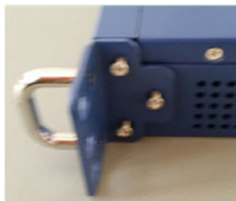
Figure 1.2 Mounting ear screws inserted but not fastened yet
