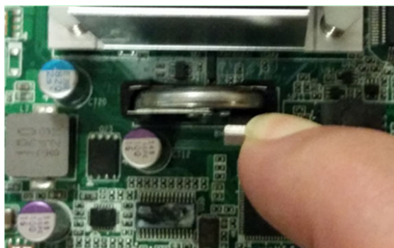
Figure 3.45 Unlocking the battery
