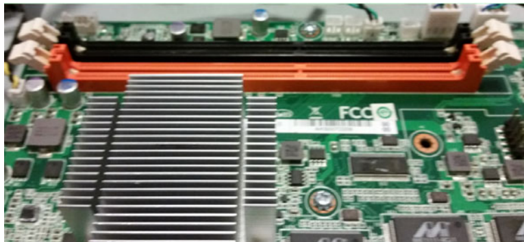
Figure 3.41 Opening DIMM latches
