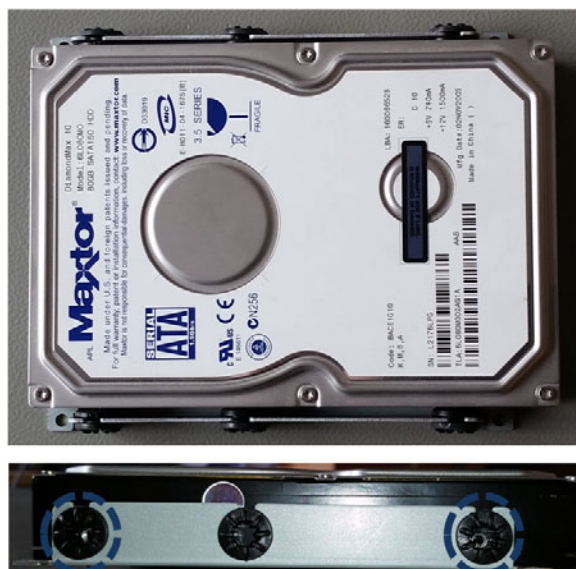
Figure 3.26 Carrier plate and HDD alignment
