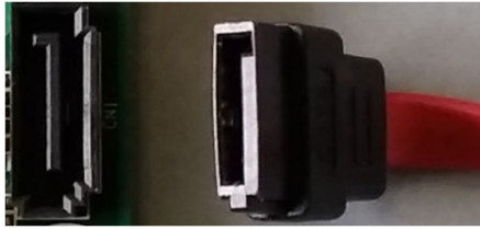
Figure 3.31 SATA Connector keying
