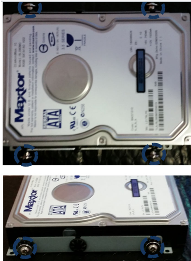
Figure 3.27 Screw insertion and fastening
