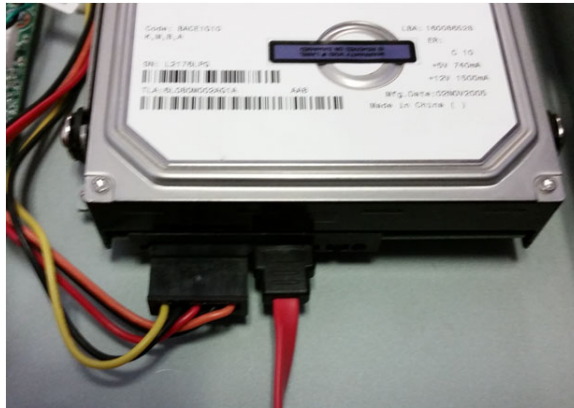
Figure 3.32 HDD Power cable
