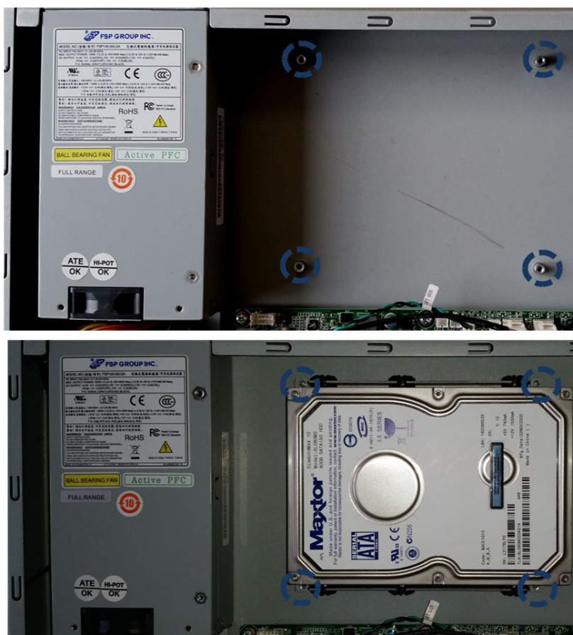
Figure 3.29 Insertion of the carrier into the chassis
