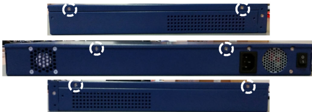
Figure 3.21 Top cover screw locations ( left/rear/right)
