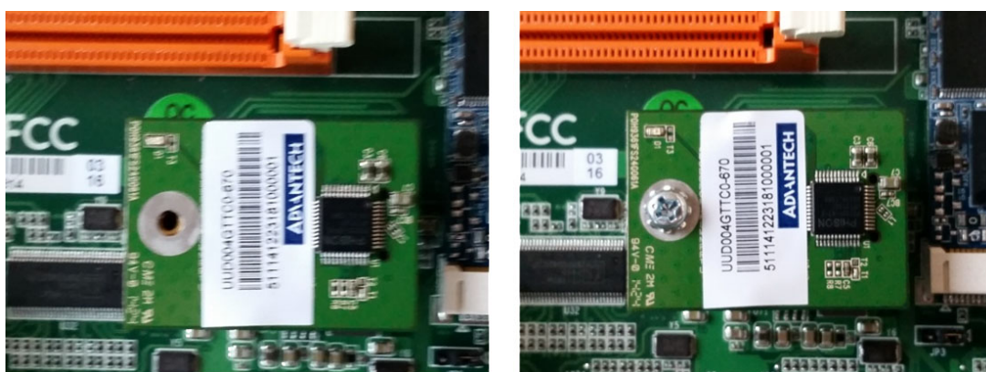
Figure 3.36 USB DOM mounting
