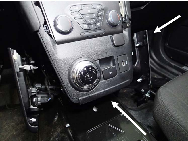
Reattach lower center and side trim panels.
