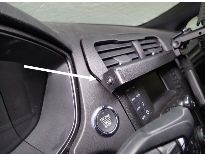
Attach frame to upper driver side support bracket with 10-32 x 1/2" screw and star washer.
