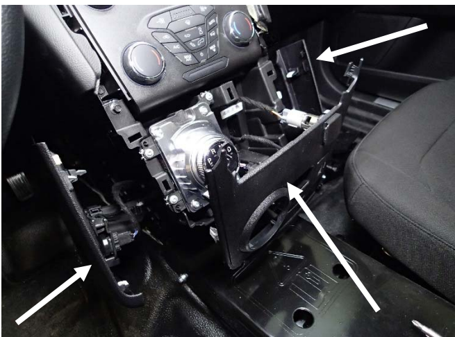
Carefully partially remove lower center and side trim panels. It is not necessary to completely remove and unplug panels.
