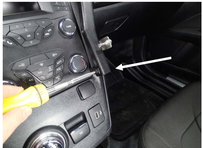
Attach frame to lower passenger side support bracket with 10-32 x 1/2" screw and star washer.
