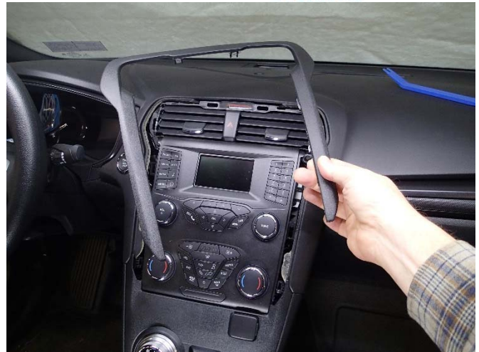
Carefully remove upper center trim bezel using plastic panel tool.
