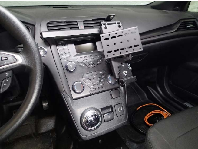
Place DMM main frame onto the support brackets.
