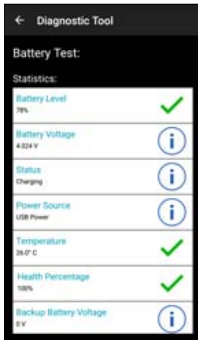
Figure 88 Battery Subsystem Details
