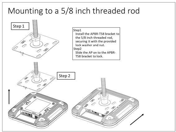
The bracket attaches to a rod that is 5/8"-11.
