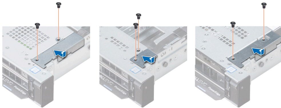
Figure 110. Installing the cable cover
