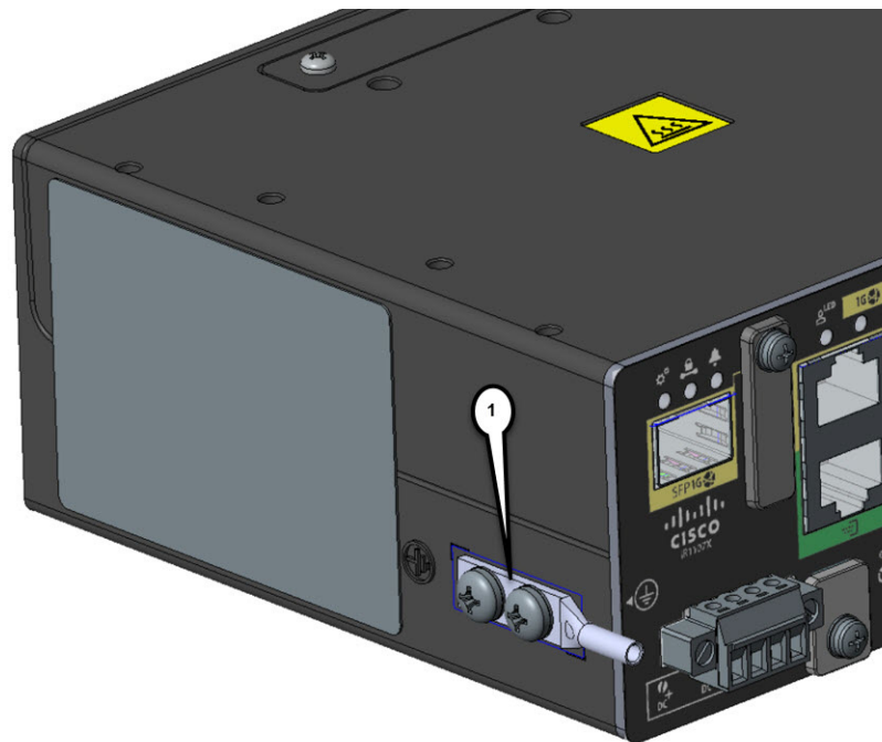
Figure 7 Chassis Ground Connection Points
