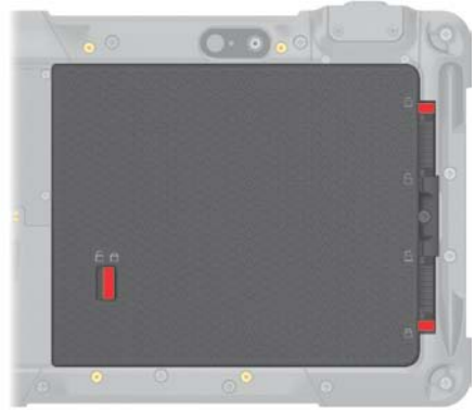
Incorrect (revealing red part)
