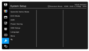
• **Splendid Demo Mode**: Splits the screen into two for Splendid modes comparison. (DCI-P3 Mode and sRGB Mode only)
