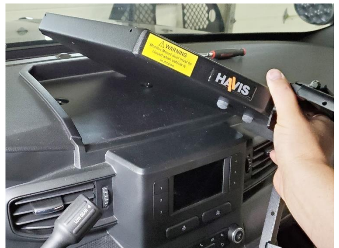
Place DMM tray assembly into OEM plastic tray and attach using M5 x 30mm bolts and 1/4" washers. (8mm socket)
