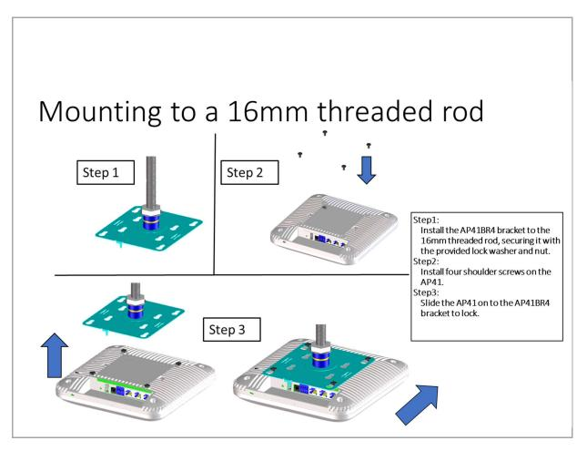
In a wall mount installation, please use screws that have a 1/4in. (6.3mm) diameter head with a length at least 2 in. (50.8mm). The AP41BR4 attaches to a rod that is M16-2.
