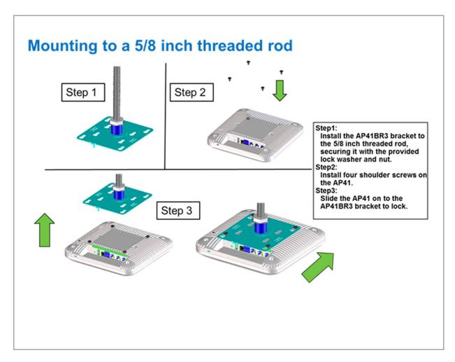
In a wall mount installation, please use screws that have a 1/4in. (6.3mm) diameter head with a length at least 2 in. (50.8mm). The AP41BR3 attaches to a rod that is 5/8''-11.
