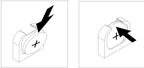
Figure 48. CMOS battery installation
