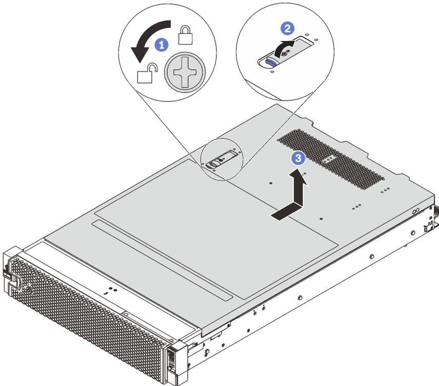
Figure 45. Top cover removal
