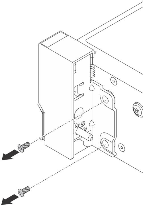
*Figure 38. Screws removal*
