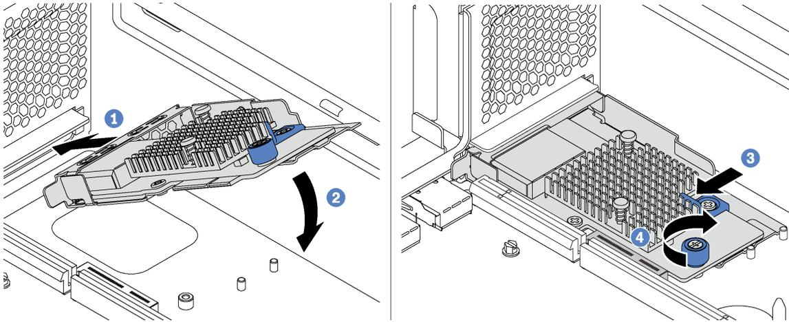
Figure 99. LOM adapter installation
