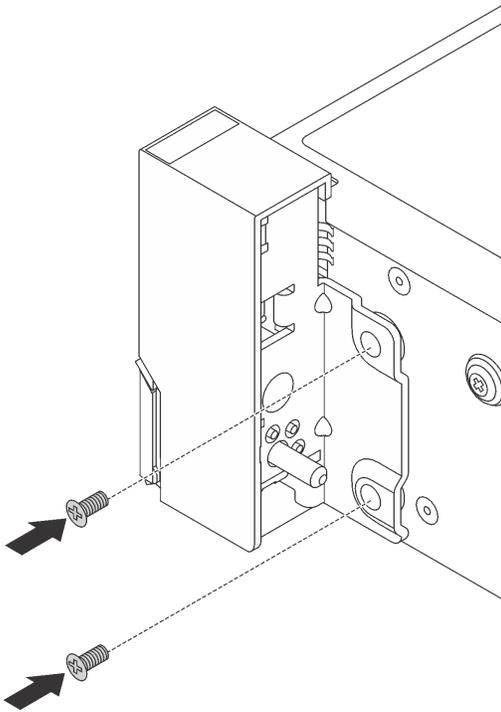
Figure 41. Screws installation
