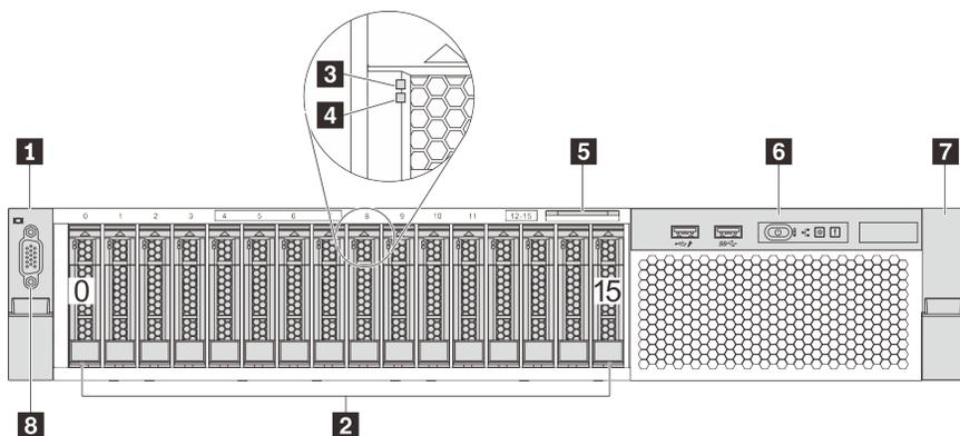
Figure 5. Front view of server models with sixteen 2.5-inch drive bays
