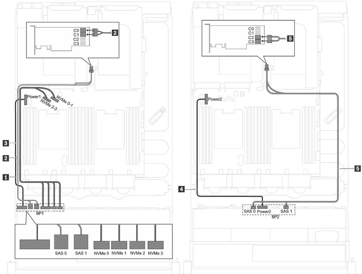
Figure 23. Cable routing for server models with twelve 2.5-inch SAS/SATA drives, four 2.5-inch SAS/SATA/NVMe drives, and one 16i RAID/HBA adapter
