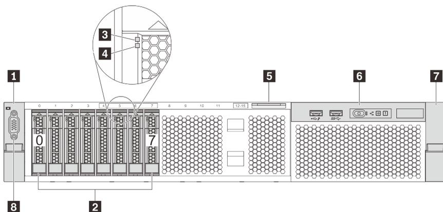
Figure 4. Front view of server models with eight 2.5-inch drive bays
