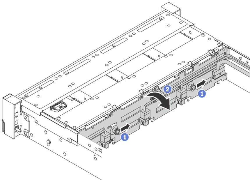
*Figure 73. 3.5-inch-drive backplane removal*
