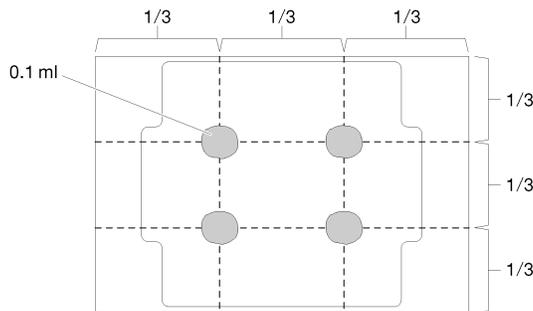
Figure 124. Thermal grease application
