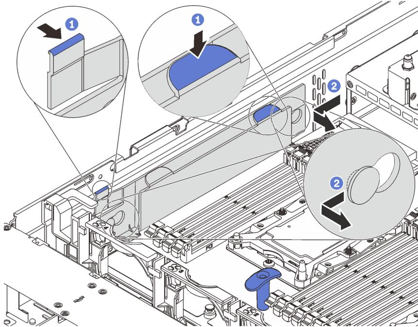
Figure 127. Cable holder removal
