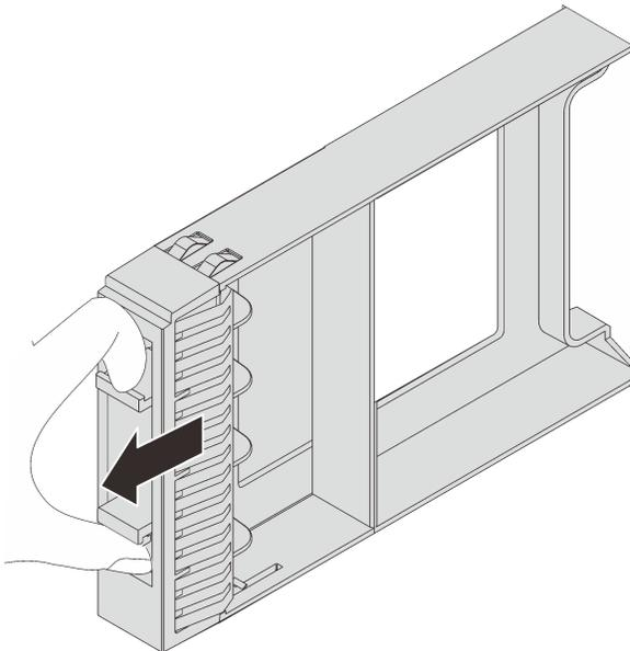
Figure 64. 2.5-inch drive filler removal
