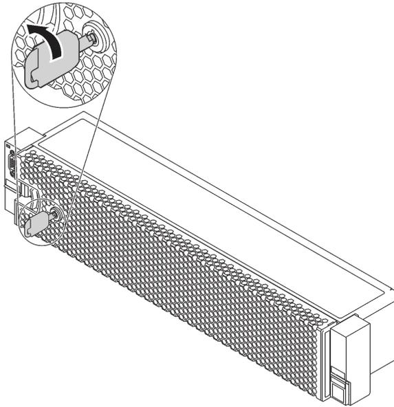
Figure 34. Locking the security bezel
