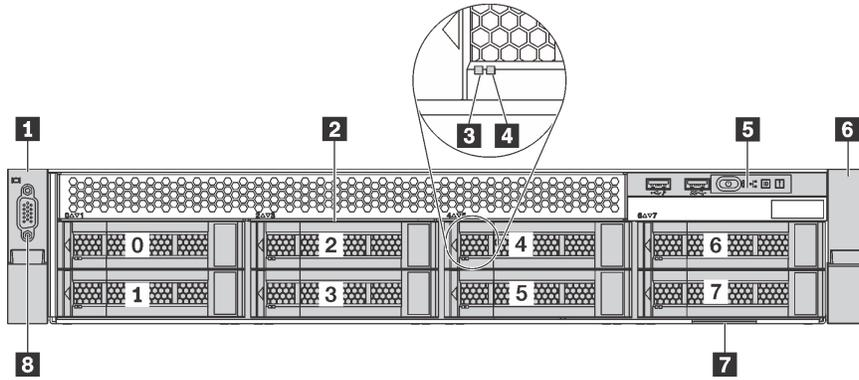
Figure 6. Front view of server models with eight 3.5-inch drive bays
