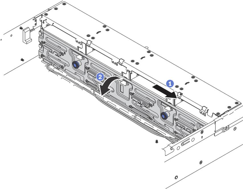
Figure 75. 3.5-inch simple-swap-drive backplate assembly removal
