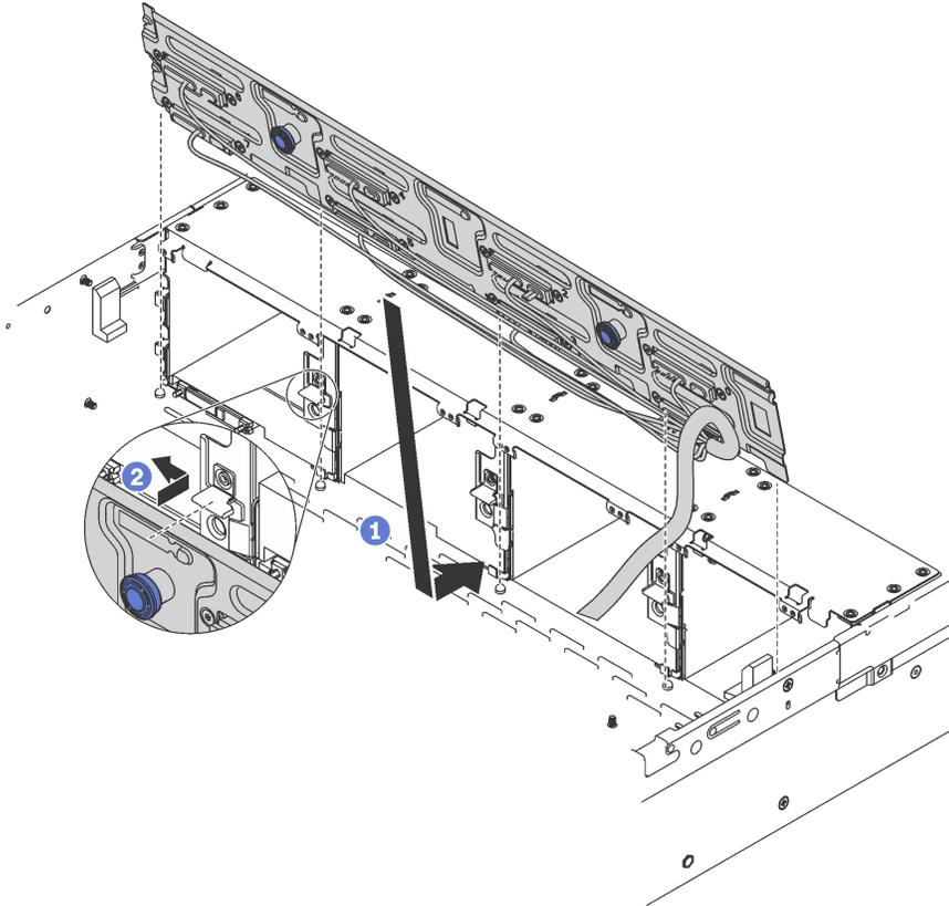
Figure 76. 3.5-inch simple-swap-drive backplate assembly installation
