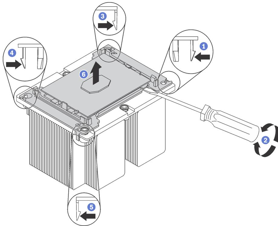
Figure 121. Separating a heat sink from a processor
