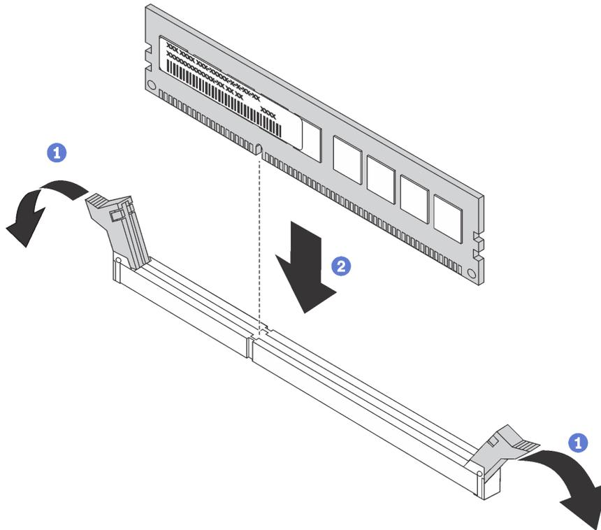
Figure 78. Memory module installation
