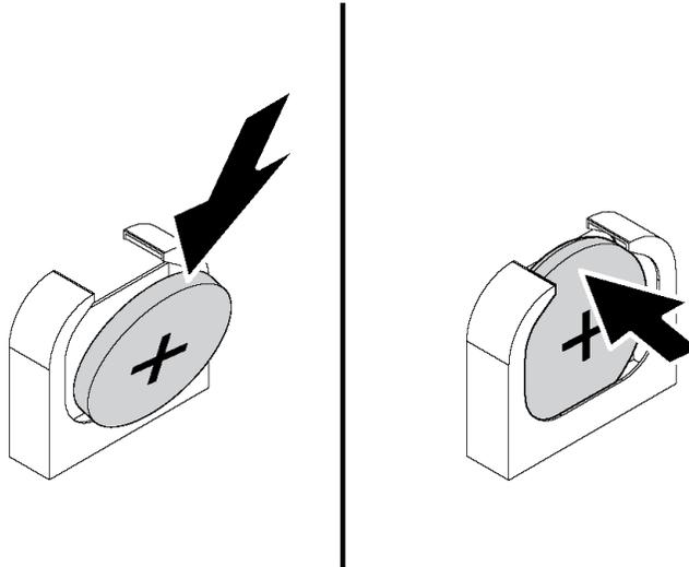
Figure 81. CMOS battery installation
