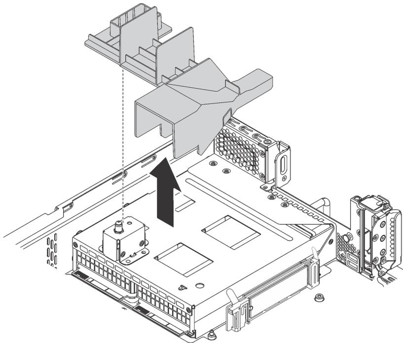
Figure 102. M.2 drive air baffle removal
