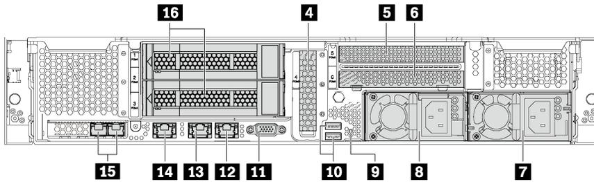
Figure 11. Rear view of server models with two rear drive bays and three PCIe slots
