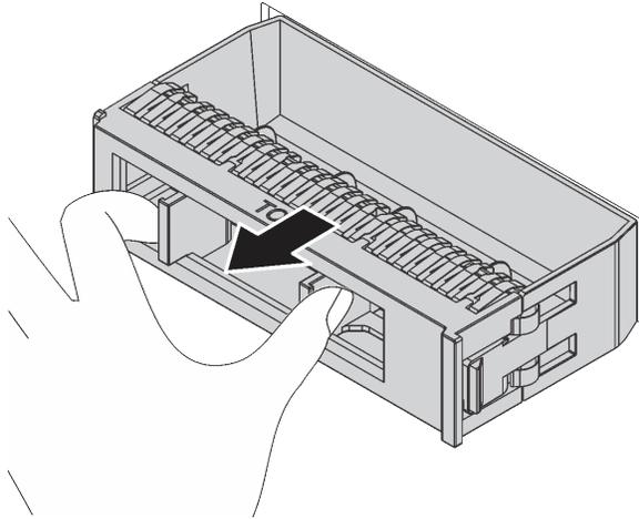
Figure 65. 3.5-inch drive filler removal
