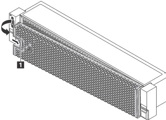
Figure 31. Security bezel removal
