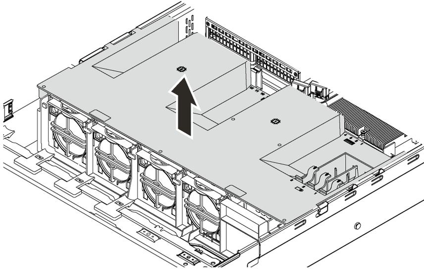
Figure 50. Air baffle removal
