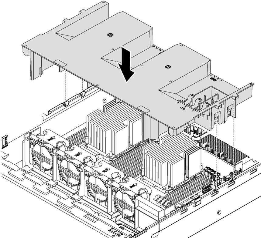
Figure 51. Air baffle installation
