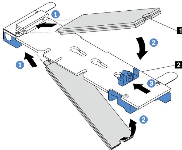
Figure 107. M.2 drive installation
