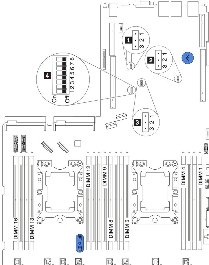
Figure 15. System board jumpers
