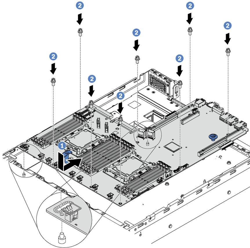
Figure 129. System board installation
