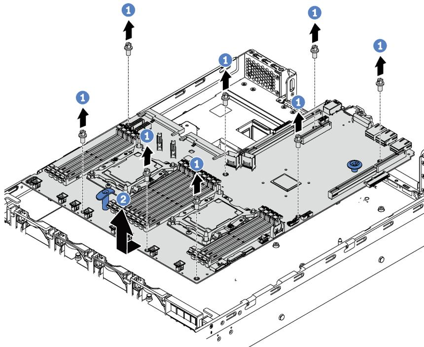
Figure 128. System board removal
