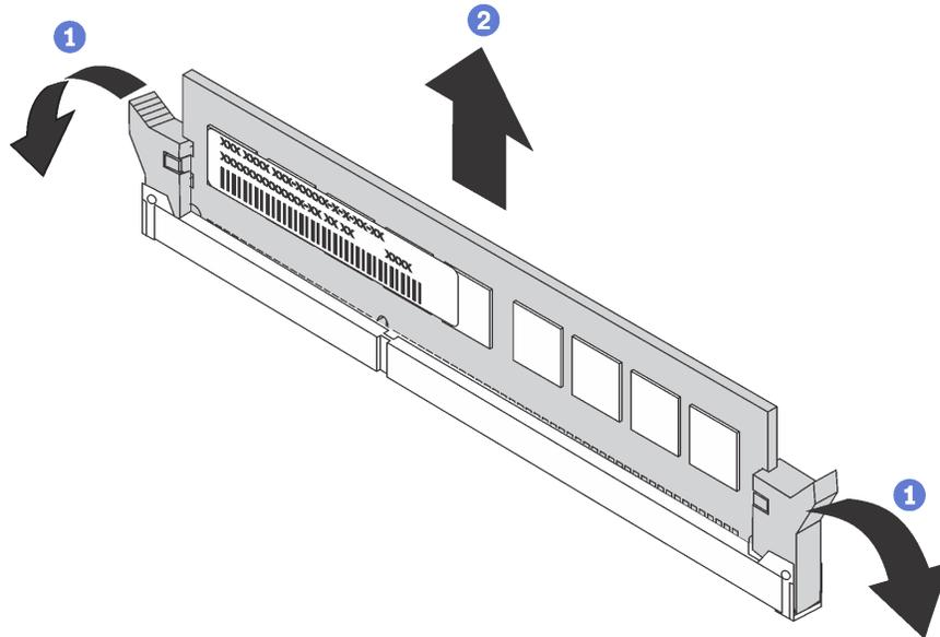
Figure 77. Memory module removal
