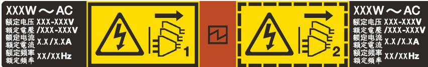
Figure 111. Hot-swap power supply label on the cover
