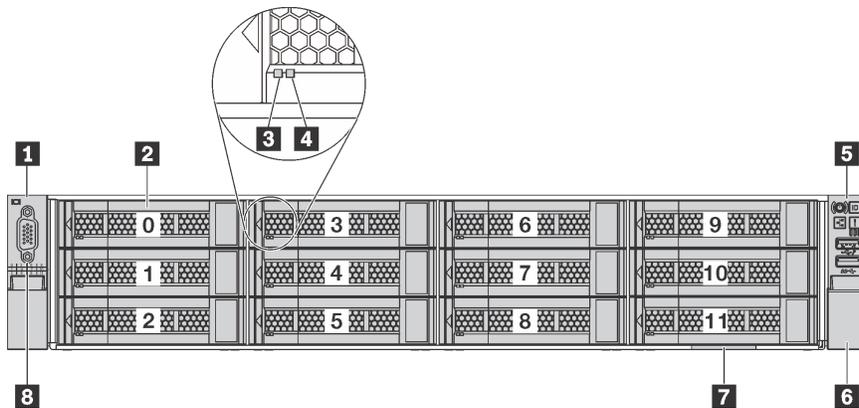
Figure 7. Front view of server models with twelve 3.5-inch drive bays
