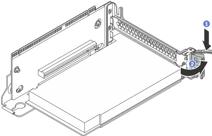
Figure 89. Opening the PCIe adapter retention latch
