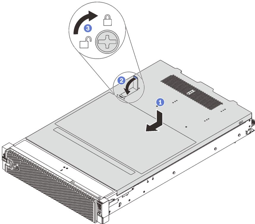
Figure 46. Top cover installation
