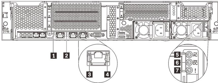
Figure 12. LEDs on the rear of the server
