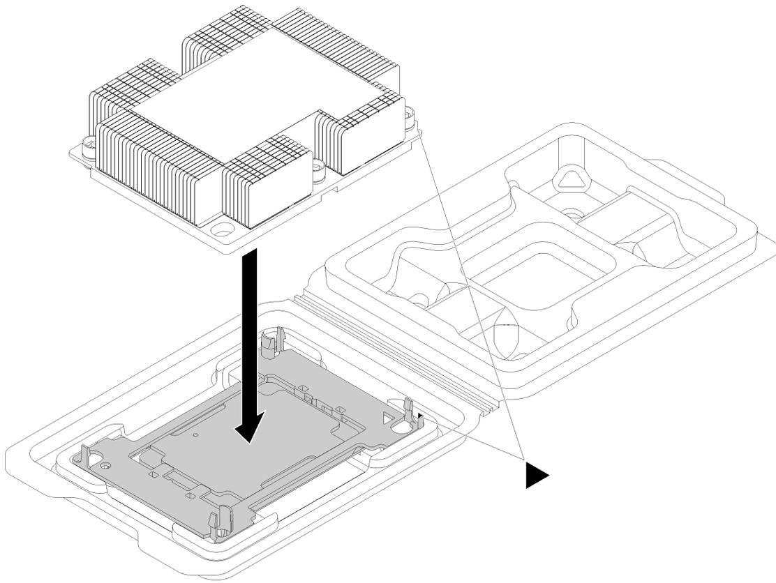
*Figure 125. Assembling a PHM in the shipping tray*
