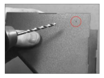
Step 2. Install supplied tamper resistant screw through drilled hole into tab on back.
