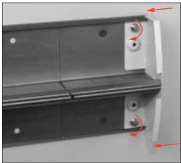
Step 3. Snap Trim Piece from DS4010B down onto End Fitting from top covering DS4000C Raceway Cover sections and snapping into slots on End Fitting.
