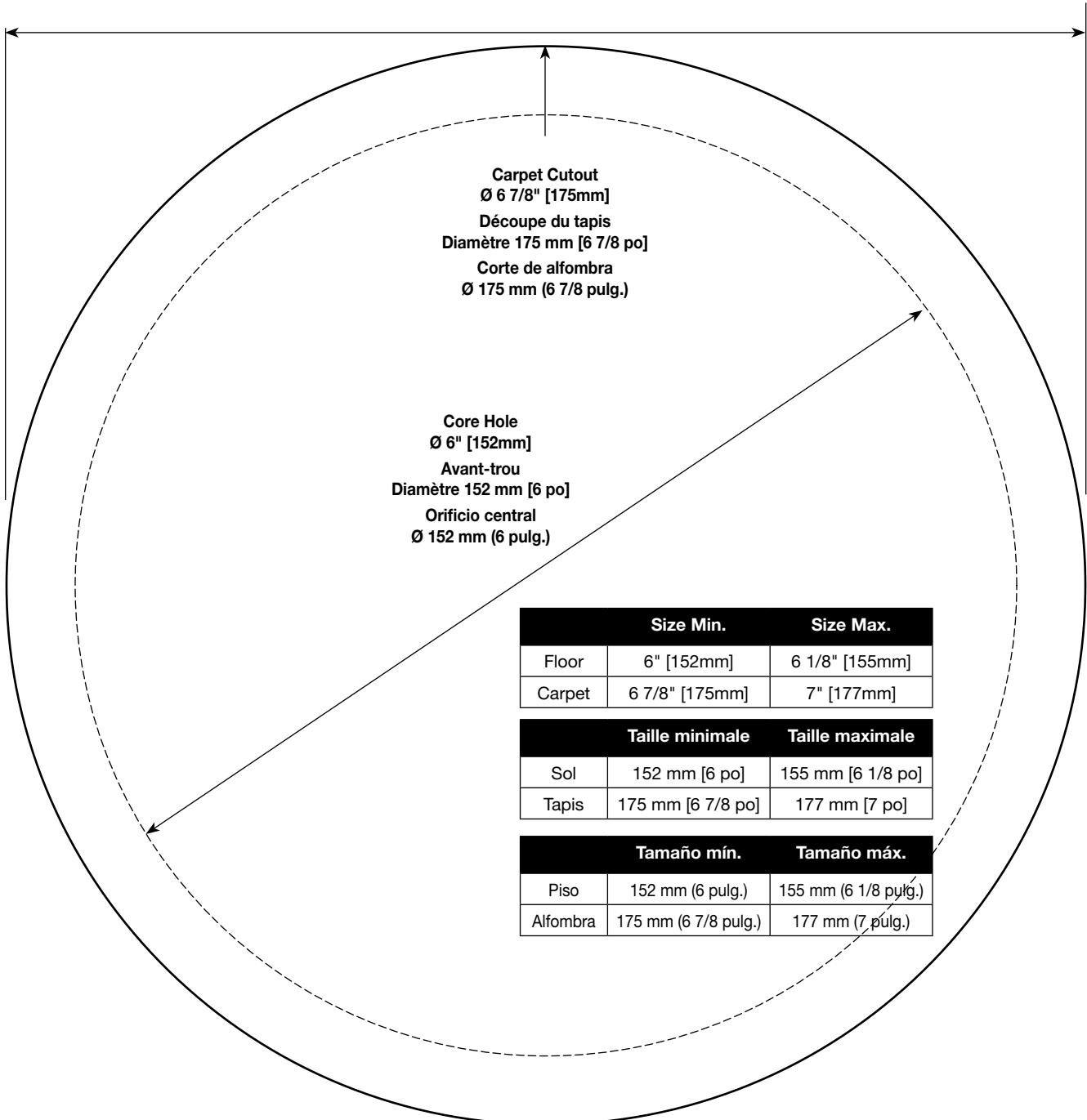
**NOTE:** When printing copies of this template, please be sure template has scaled correctly and is the correct size before using it to cut the floor.
