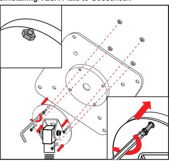
Align screw holes inside the circle on VESA plate with the screw holes on the gooseneck plate and hold together. Press screw through hole starting from gooseneck side, then attach nuts on the VESA side.
