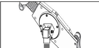
Locate the 4 screws connecting the tablet holder to the gooseneck on the circular plate.
