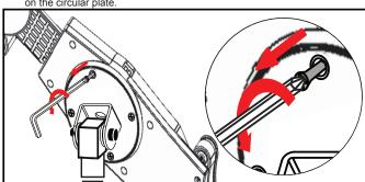
2. Use a Phillips screwdriver to unscrew screw on the circular connection plate.
