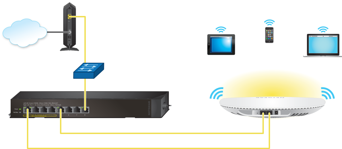
Figure 7. Link aggregation connection
