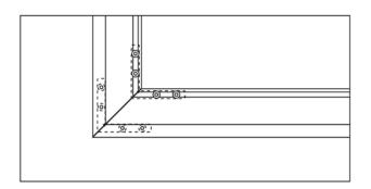
Note: You may have to loosen and adjust the brackets and frame pieces. It will help to leave the screws loose until perfect right angles are formed, then tighten the screws securely.
