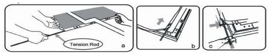
**Step 7.** Insert the *Springs* (*B*) into the grooves of the frame. Line them up with the corresponding holes in the materials edge. Be sure the shorter hook on each spring is placed in the frame's groove, while the longer hook attaches to the material. For the correct amount of springs to place into the frame, please refer to the table listed below.
