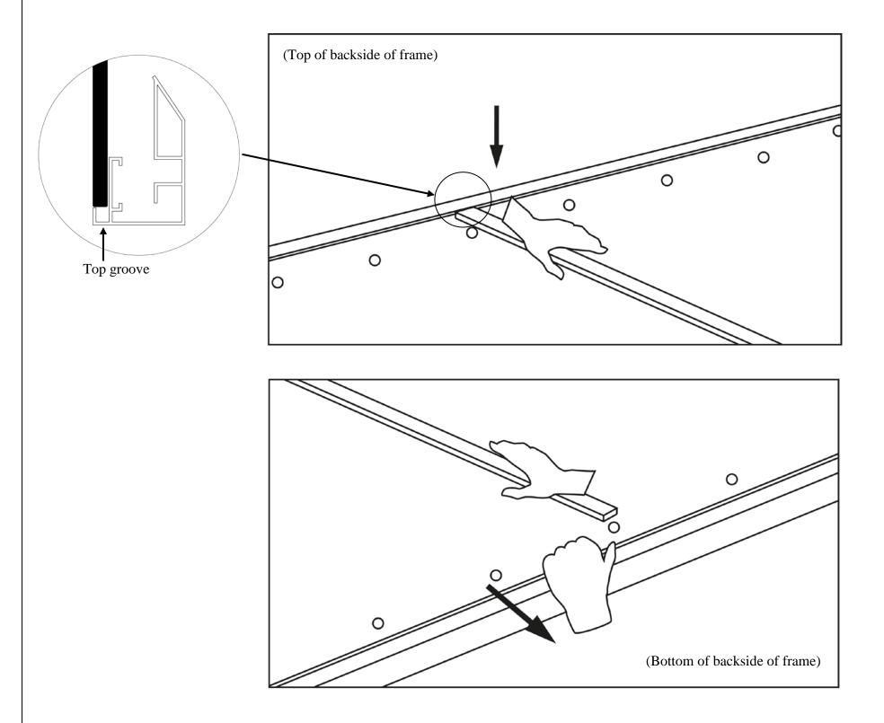
Step 10. After the *Center Support Bar* (J) secure, connect the center of the vertical portions of the material (2). **Be sure to hook the** *Springs* (B) onto the *Tension Rod* (I) to avoid damage to the screen material. Next, return to the vertical sides, securing the remainder of the springs (3). Lastly, secure the remaining springs of the horizontal sides of the screen (4).
