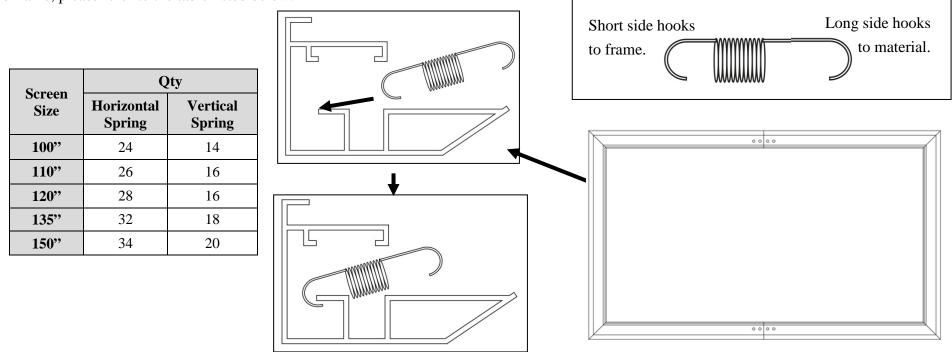
**Step 8.** With one end of the spring placed inside the groove of the frame, hook the *Spring (B)* through the hole located on the screen material's outer edge. **Be sure to hook the** *Springs (B)* **onto the** *Tension Rod (I)* **to avoid damage to the screen material.** Use the *Pull Hook (E)* when necessary. Attach the four corners and center horizontal sections of the material (1).
