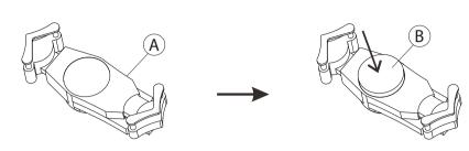
4A. Select the appropriate foam pad (B) according to the thickness of your tablet. (See table on the right for reference) Once you have your foam piece selected, peel off the sticker and with the adhesive side, face down onto the tablet and press onto the holder (A). Make sure to align foam to the center of the tablet holder where there is a small circle indication. Also foam pieces can stack as needed by the user's discretion.
