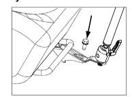
2B. Install the full assembled vehicle mount on the seat rail and screw the bolt back as shown. (Tool not included)
