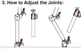
3A. Twist the screw knobs counter-clockwise to release the connection. Adjust the arm to your any preferred position & rotate back clockwise until securely tightened.
