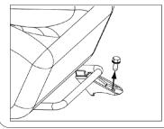
2A. Loosen the bolt (not included) of the seat rail.(seat and rail not included)
