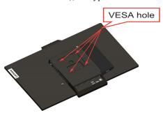
Step 5: Attach the LCD display to the wall, and follow the instructions in the wall-mounting kit.
