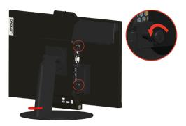
2. Push the computer from the rear as shown to disconnect it completely from the 3 in 1 cable.
