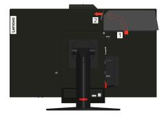
2. Screw the rear Wi-Fi antenna to the antenna connector on the rear of the computer. Then, adjust the angle of the antenna to 90 degrees.
