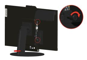
Part 3: Install the rear Wi-Fi antenna (optional).
