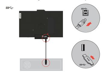
5. Connect one end of the USB cable to the USB downstream terminal on the side of the monitor, and connect the other end of the USB cable to an appropriate USB port on your
