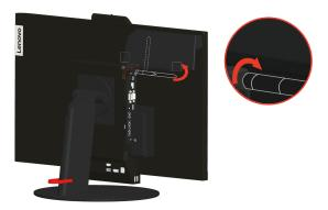
3. Pivot the cable cover as shown to the closed position.
