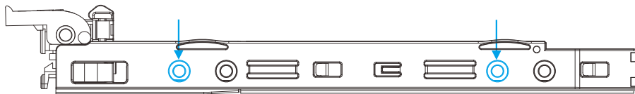
Installing a 3.5" HDD with a MUX Board (SATA drives)
