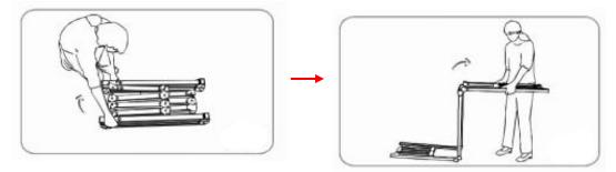
2. Next, unfold the frame until the latch on the hinge "clicks" into place. Repeat the procedure for the shorter sections, as shown below.
