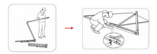
3. After making sure the legs are secure to the frame, using two people, lift the screen up in a vertical position. While the screen is in a vertical position, fold the front feet of the legs out.
