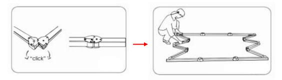
**Note:** When unfolding the frame and legs, be sure the latches on the hinges "click" into place. Please also make sure all 4 corners of the frame are at a  $90^{\circ}$  angle and the hinged support bar is straight and not bent.
