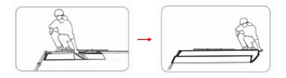
2. Once the screen material is fully extended, secure the material by snapping the buttons onto the frame studs. Fasten the buttons in the following order as shown on **Fig.1**.
