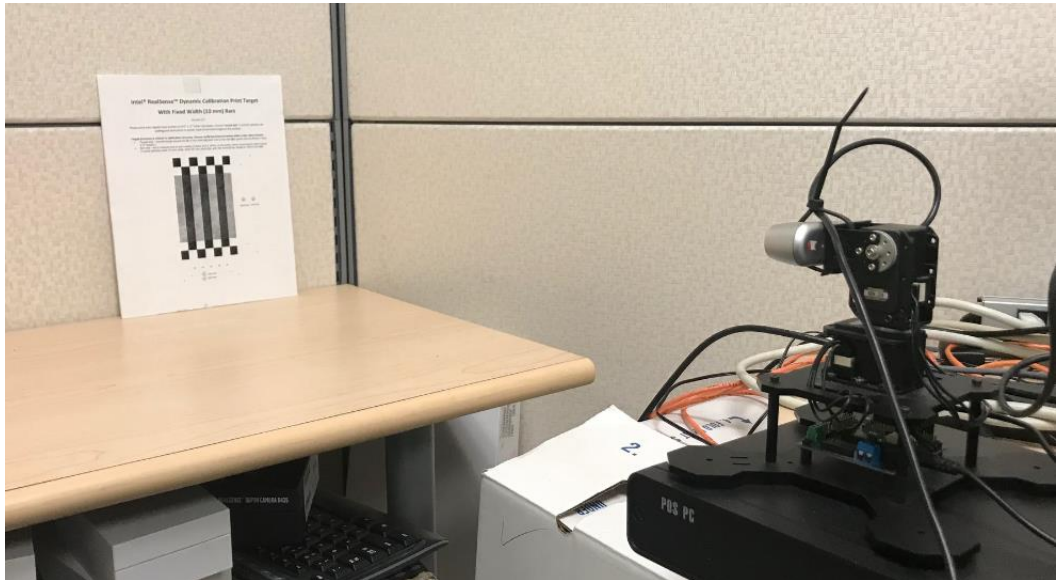
Figure 5-8 Dynamic Calibration on Robot – Sample Setup
