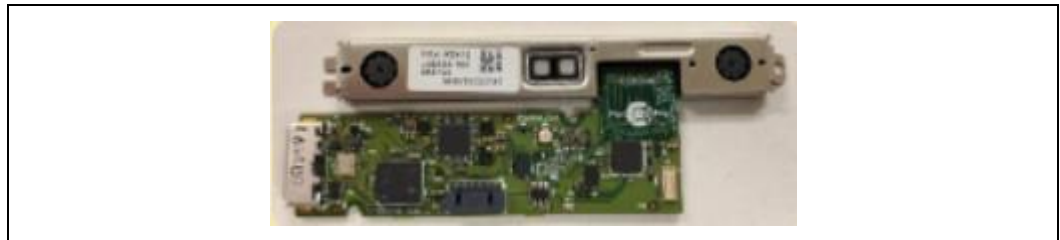
Figure 1-2. Intel® RealSense™ Depth Module D410 with Vision Processor D4 Card (Non-integrated Bare Depth Module)
