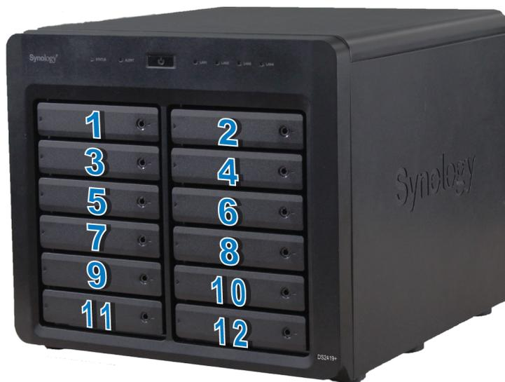
**Note:** If you want to create a RAID volume, we recommended that all installed drives are of the same size to make the best use of drive capacity.
