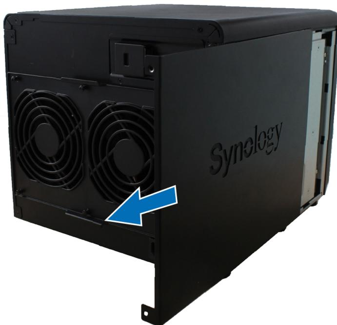
**Note:** When you remove the case, you expose sensitive internal components. Avoid touching anything other than the memory assembly when you remove or add memory.
