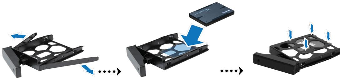
4 Insert the loaded drive tray into the empty drive bay.
