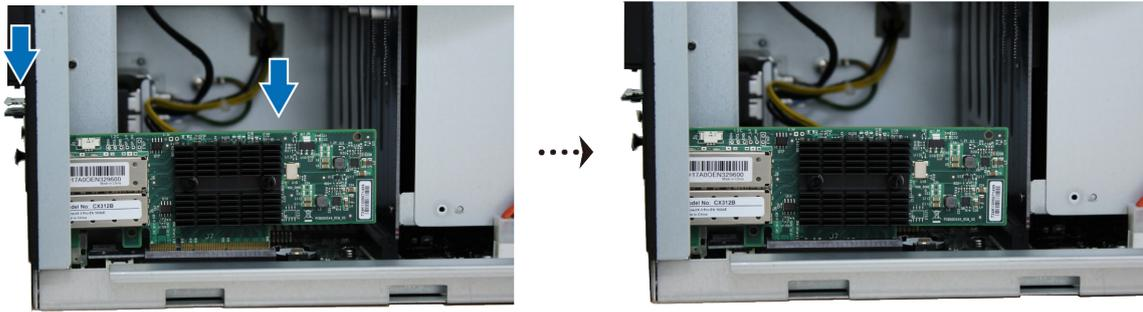
c Push back the clip to secure the newly inserted card.
