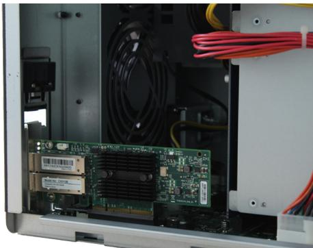
b Use two fingers with firm, even pressure to push down on the card and the bracket.
