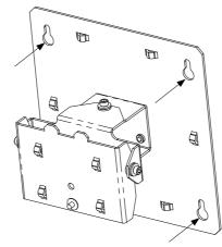
Step 3a. Install Drywall Anchor: Install one drywall anchor at each hole mark. Using a #2 Phillips head screwdriver press the anchor into the drywall while turning clockwise until it is seated flush with the wall.
