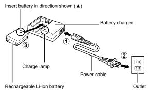
· Batteries charge in about 2 hours. Charge status is shown as follows:
