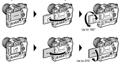
· Gently rotate the monitor within its range of motion. Attempting to rotate the monitor beyond the limits shown below could damage the connectors.
