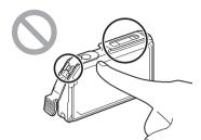
• Do not shake the ink tank with the ink supply opening down. Ink leaking from the ink supply opening could stain your clothes or the area around the printer.
