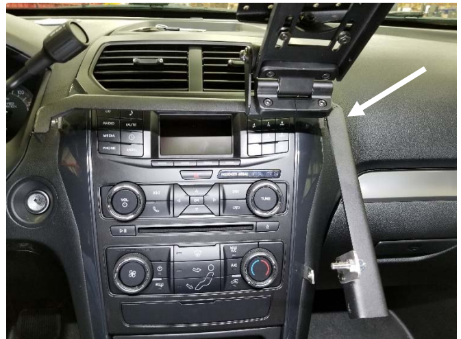
Place DMM frame onto the support tabs and attach the upper passenger side corner using 10-32 x 1/2" screw and star washer.
