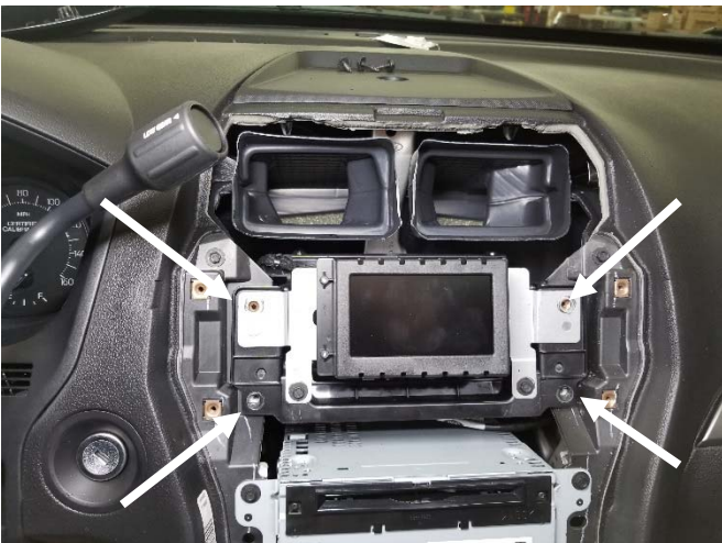
Remove (4) 7mm head screws
