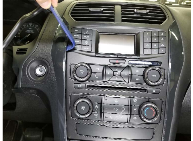
Carefully remove driver and passenger side trim bezels using plastic panel tool.
