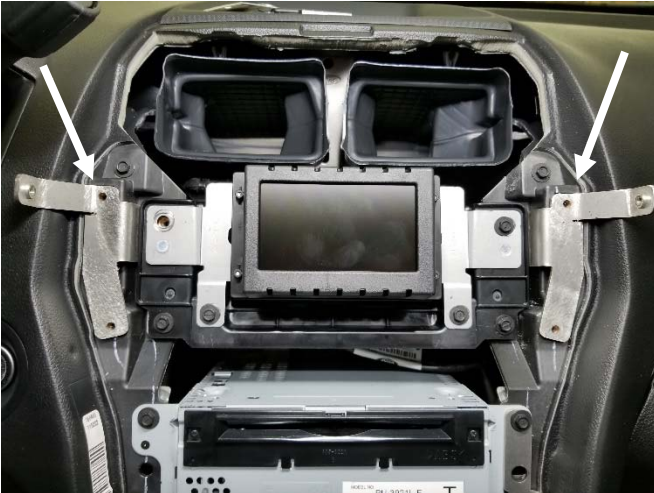
Place driver and passenger upper support brackets in vehicle and attach using OEM fasteners. Torque to 3 Nm (27 in-lbs.)
