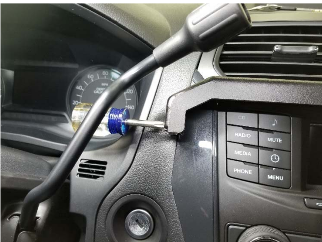
Attach the upper driver side corner using supplied 10-32 x 1/2" screw and star washer
