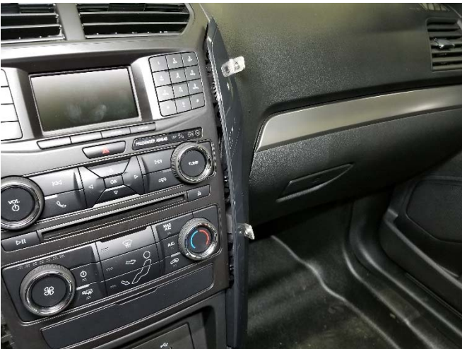
Reattach trim bezels allowing the support brackets to sit between the bezel and the dash.
