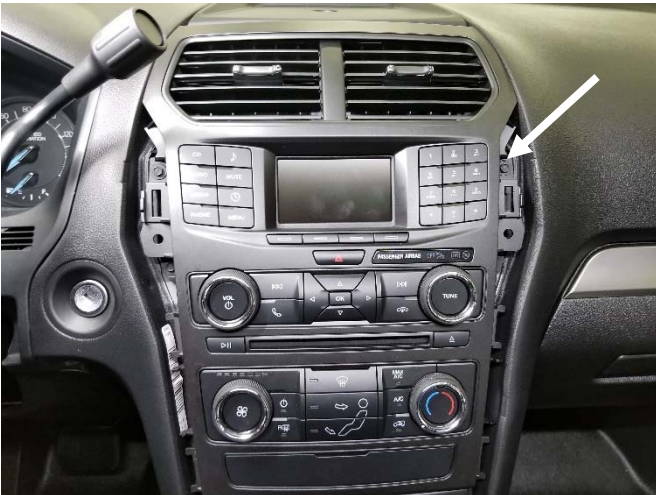
Remove screws holding center panel. Unplug and remove center control panel.
