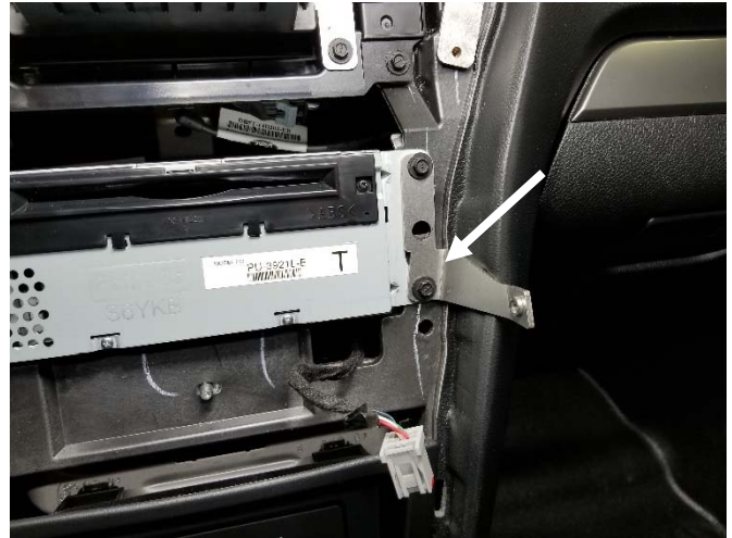
Attach lower support bracket to dash using OEM 7mm head fasteners Torque to 3 Nm (27 in-lbs.)
