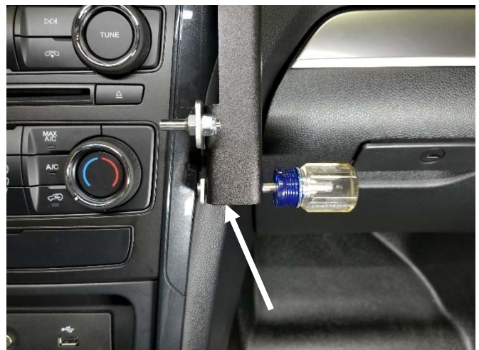
Attach the lower passenger side with 10-32 x 1/2" screw and star washer. Access hole in the frame.
