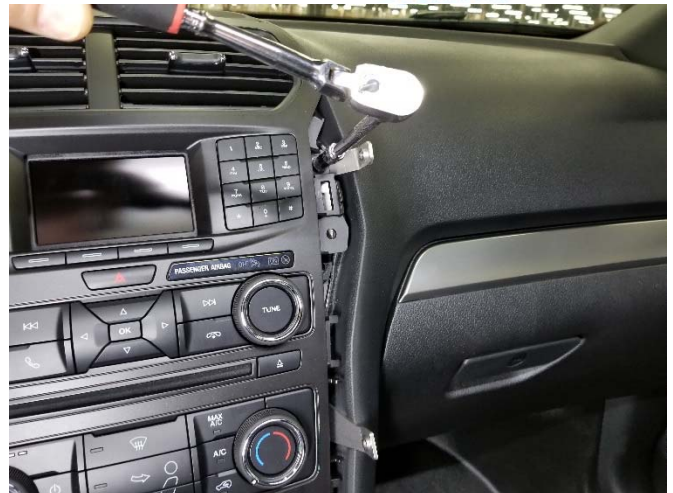
Reattach center control panel Torque to 3 Nm (27 in-lbs.)
