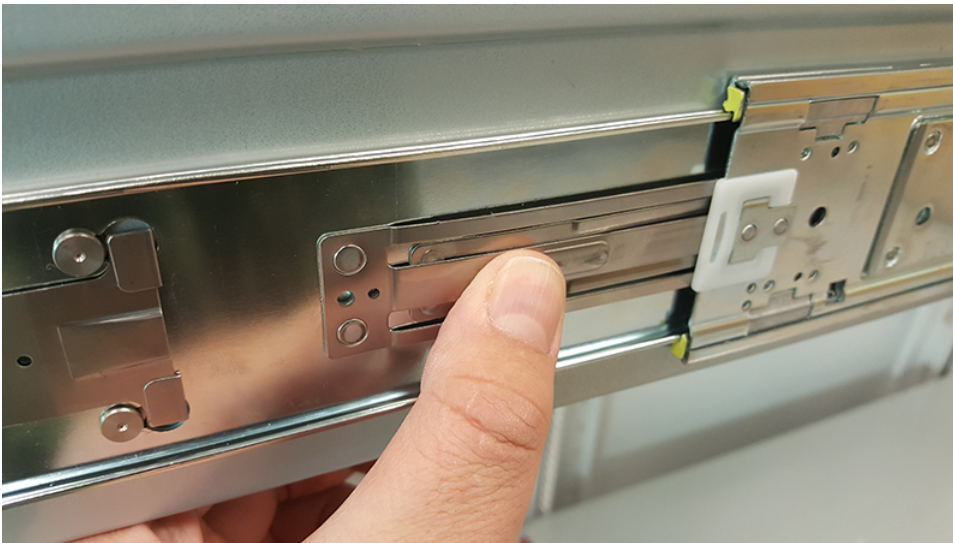
Figure 299: Inner Rail Safety Latch Release
