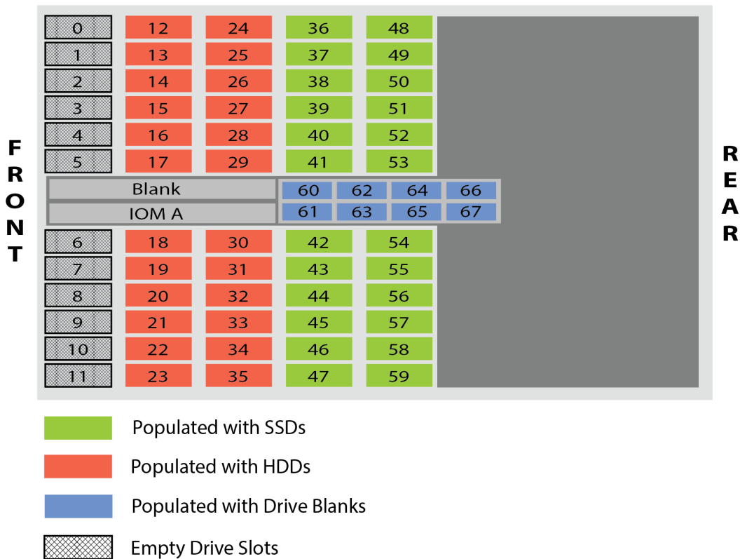
Figure 445: Minimum HDD and Maximum SSD Partial Population
