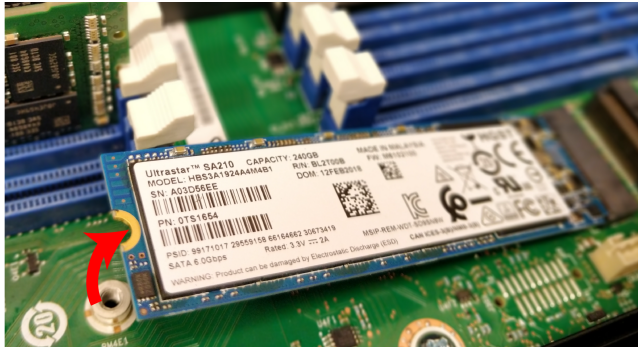
Figure 201: Uninstalling the M.2s
