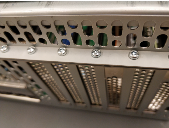
Figure 224: Add-In Card Screws
