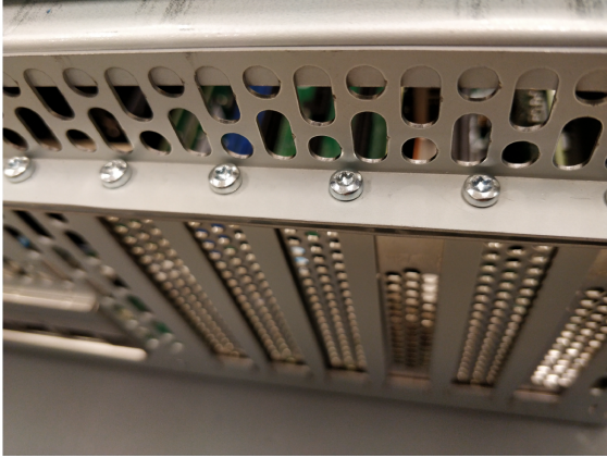
Figure 315: Add-In Card Screws
