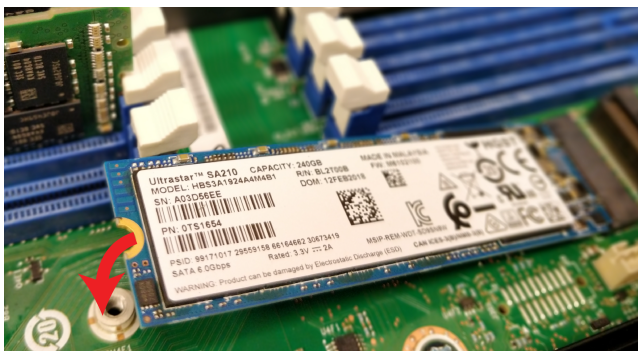
Figure 203: M.2 Install (Top)
