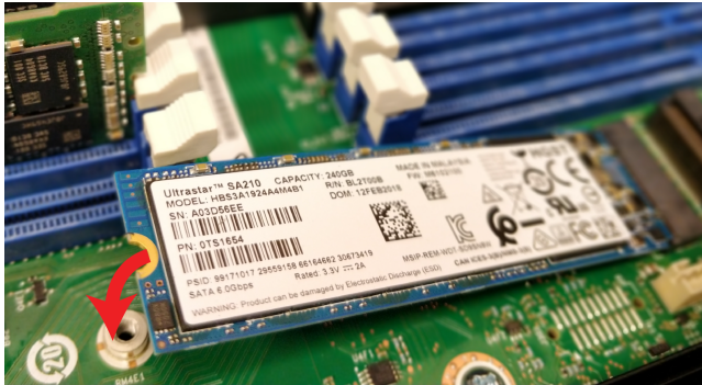
Figure 330: M.2 Install (Top)
