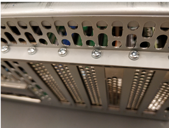
Figure 231: Add-In Card Screws
