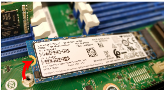
Figure 314: Uninstalling the M.2s
