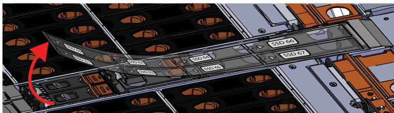
Figure 351: Lift the Center Channel Flap
