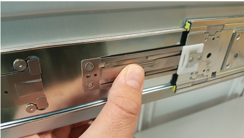
Figure 112: Safety Latch Release
