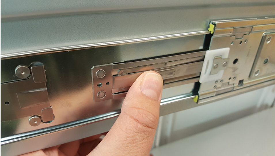
Figure 111: Inner Rail Safety Latch Release
