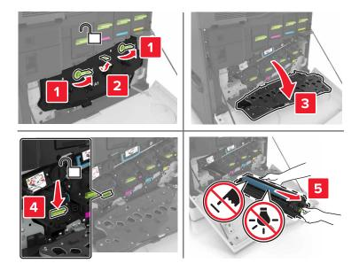
Remove the photoconductor unit.
