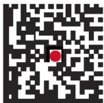
Figure 2-9 DS36X8-DP and DS36X8-DPA Aiming Pattern
