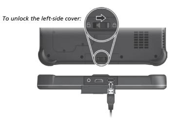
Select models have a second USB port, which supports USB 2.0 (transfer rate is 480 MB/s).
