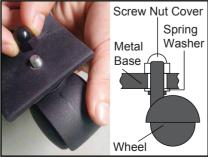
Place the screw bolt from each wheel through the metal base, then place a nut cover over the top of each. Screw down clockwise by hand, then use wrench to tighten
