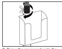
2. Screw the gooseneck onto the metal connection of the pole by turning clockwise. Be sure that the battery case is on the opposite side of the pole as the Y screw.
