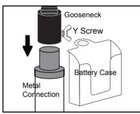
1. Place battery case over top of metal connection. Note: if Y screw is already in, unscrew before attaching gooseneck.
