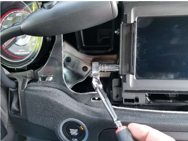
Repeat process for driver side and tighten hardware.
