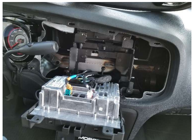
Repeat process for both sides. Make sure brackets fit around radio snug.
