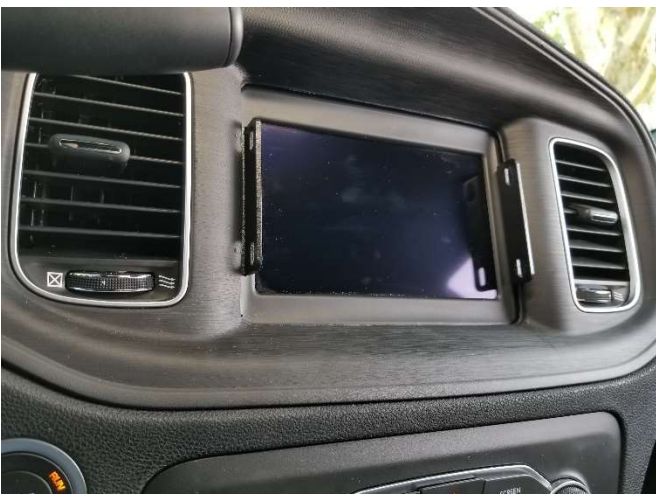
Make sure the side mounting brackets are even along the dash and the dash is fully seated back into place.
