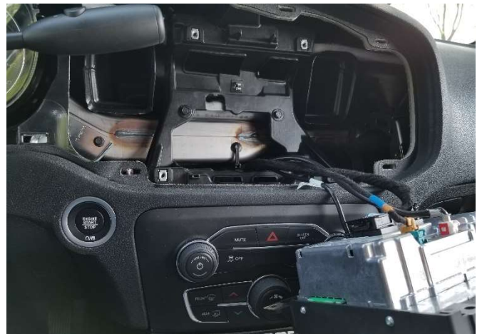
Temporarily remove radio touch screen.
