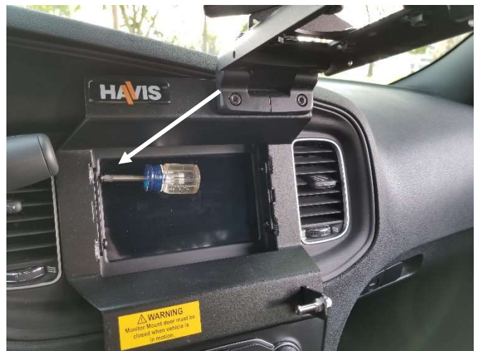
Attach main C-DMM-3005 frame to the side support brackets using 10-32 x 3/8" screws and star washers.
