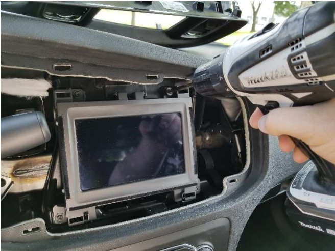
Reinstall the radio touch screen using the previously removed OEM hardware.
