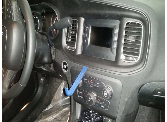
Gently pry along the dash with a flat blade panel removal tool. Slowly working along the frame.
