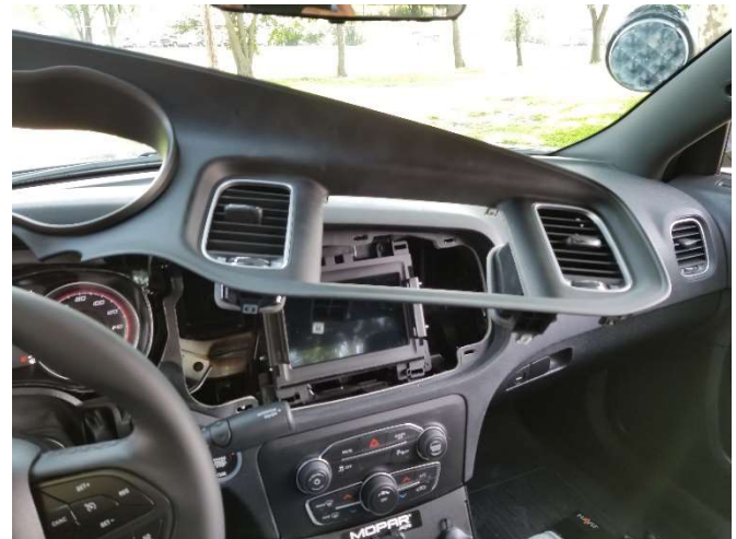
Carefully reinstall previously removed dash panel.
