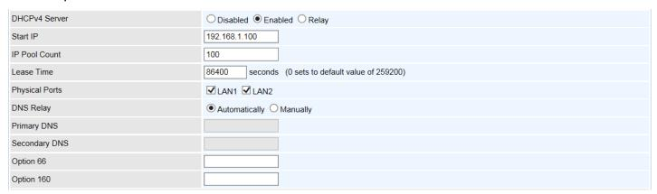
**DHCPv4 Server:** If set to **Enabled**, your MX-200Ae can assign IP addresses, default gateway and DNS servers to the DHCP client.
