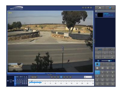
8. Use the mouse scroll to digitally zoom in and out from a single channel display.
