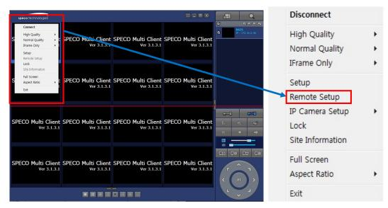
Then the setup window is displayed. The specified menu screen is displayed on the upper left of the screen. Enter the password of the NVR when prompted. (NOTE: The Password set on initial booting)
