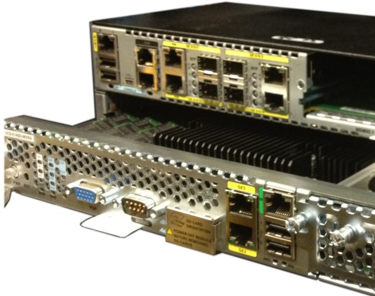
Figure 7: Double-Wide E-Series Server in a Cisco ISR 4000 series
