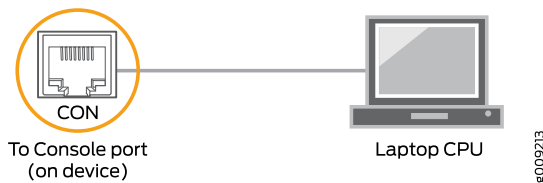
Figure 35: Connecting the NFX150 Device Directly to a Management Console
