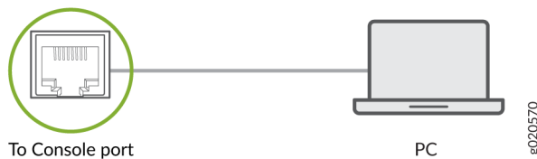
Figure 27: Connect a Device Directly to a Management Console
