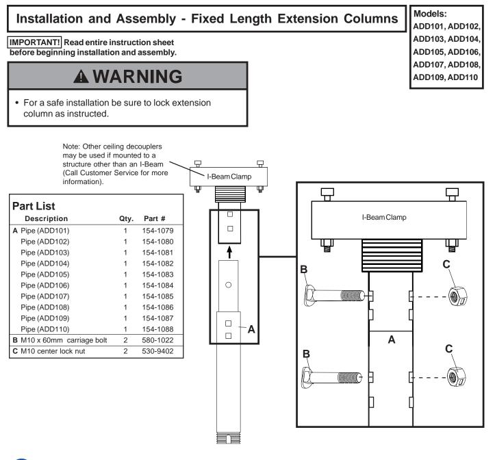
Follow directions supplied with mounting bracket for attaching to threaded end of column. Align slot with one hole inside of threaded fitting. Lock extension column with one M5 x .8" x 10mm phillips screw supplied with mount column attaches to.
