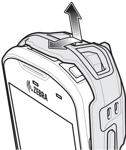
Figure 157 Lift Boot Over Device
