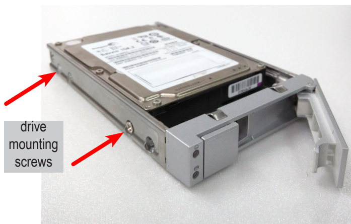
2.5" drive carrier with HDD, 'left' side with HDD undercarriage exposed
