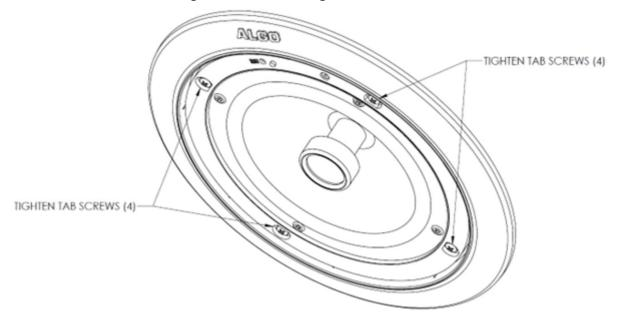
2. After installation and testing, gently work the speaker grill into its friction fit position and ensure it is evenly flush with the housing around the edge. The speaker grill is intentionally tight to prevent falling from the ceiling.
