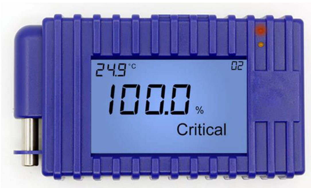
FIGURE 4-3: EXAMPLE OF SENSOR IN CRITICAL STATE (RED LED BLINKING)
